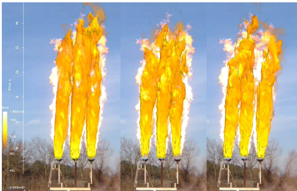
Figure 9 – Comparison of Predicted and Measured Flame Shape for the 3-Flare Test (sequential predicted images overlaid to test flame)
